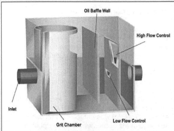
Stormwater 360 Hydrodynamic Separator. SOURCE: EPA (2005c)
