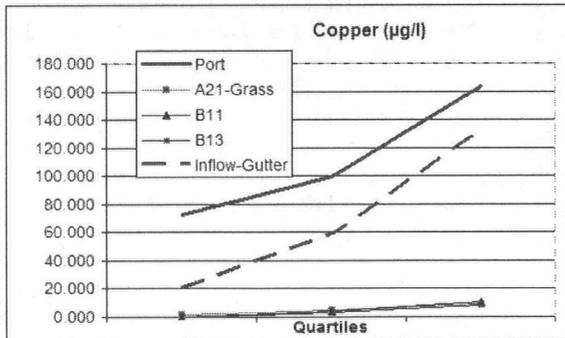
FIGURE 5-36 Copper measured at various locations. The three quartiles correspond to the 25<sup>th</sup>, 50<sup>th</sup>, and 75<sup>th</sup> percentile value of all data collected. A21 is a lysimeter location under the surrounding grass, while B11 and B13 refer to locations that are one foot and four feet under the infiltration bed, respectively. SOURCE: Reprinted, with permission, from VUSP. Copyright by VUSP.
